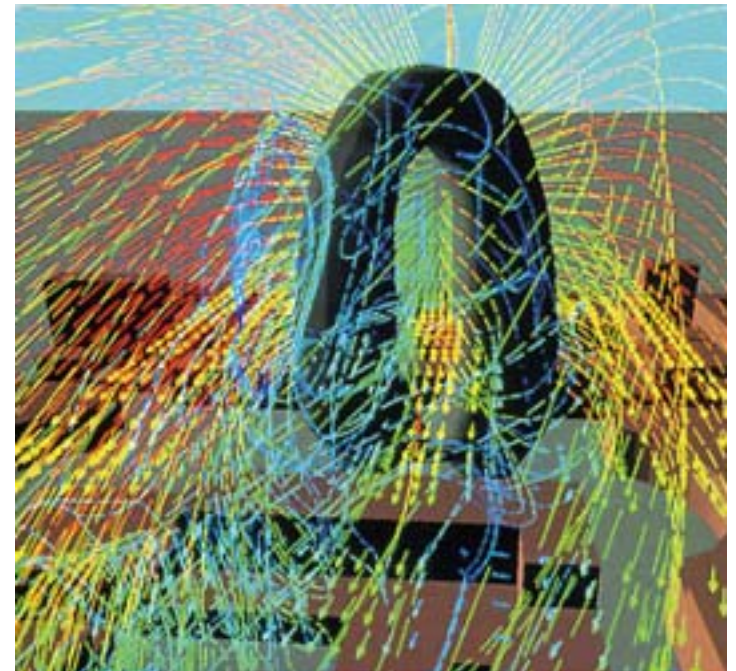
2.34. The CFD analysis of wind flows for Project ZED (1995), London, UK, architect Future Systems.
